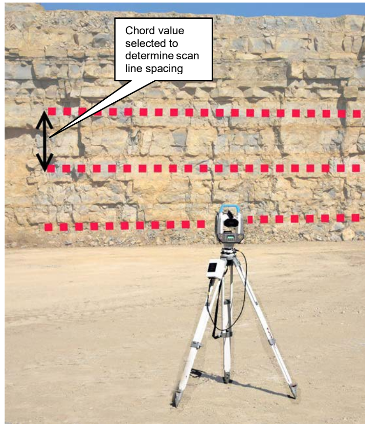
Figure 46 FastScan with Chord increment selected
