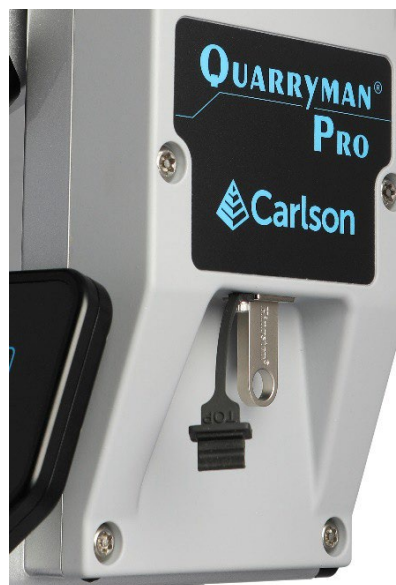
Figure 17 USB drive attached to the Quarryman Pro
