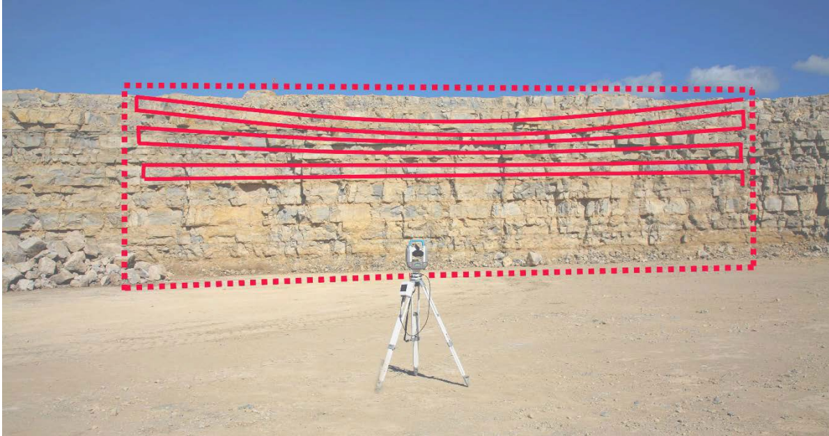
Figure 43 'Curved' horizontal scan lines
