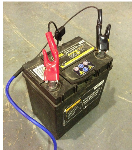
Figure 14 Crocodile clip DC cable (left) - attached to a 12 V battery (right)
